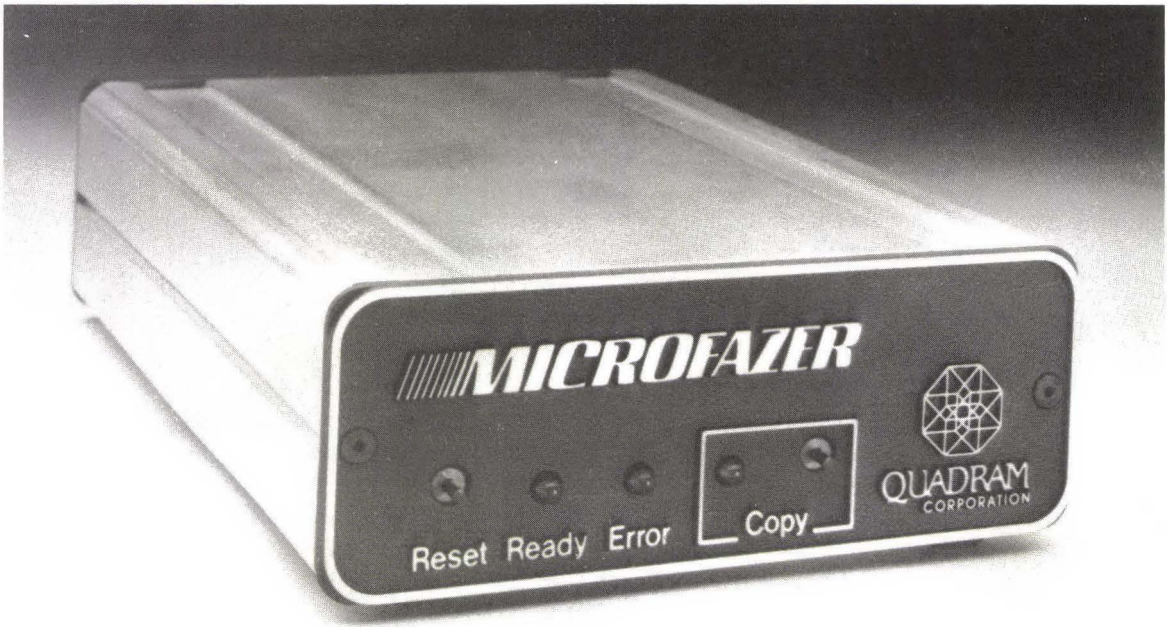
Fig. 20-5. The Microfazer buffer is available in several memory configurations, including 256K and 512K (courtesy of Quadram Corporation).
